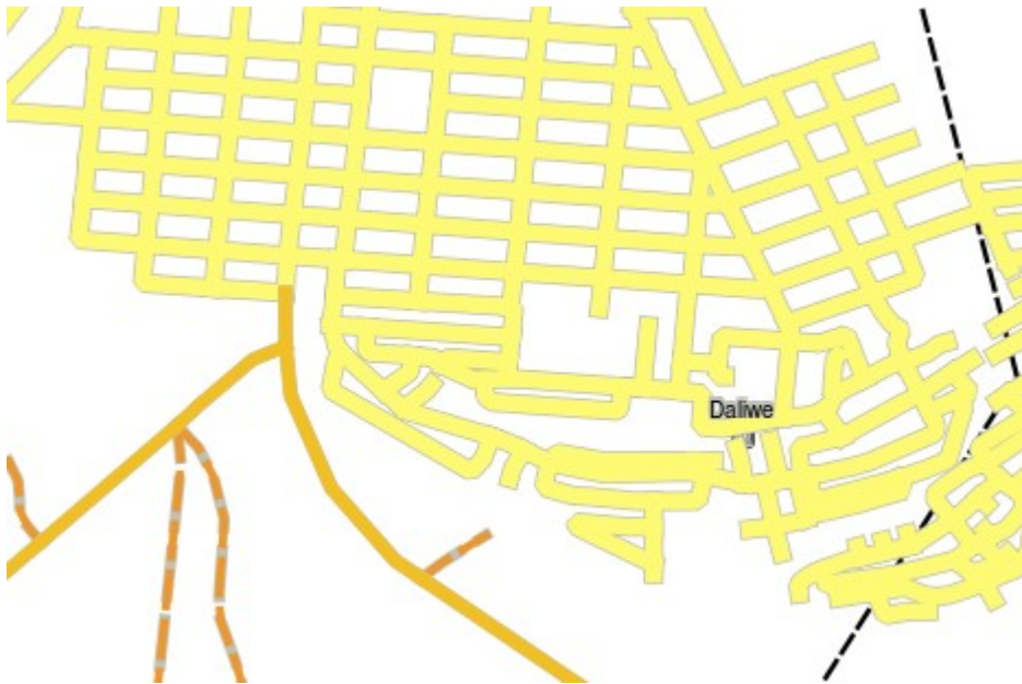
Illustration 14: A roads vector layer symbolised using a unique value per road type.
